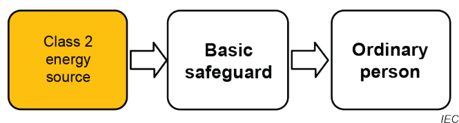
Figure 10 – Model for protection of an ordinary person against a class 2 energy source
