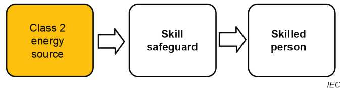
Figure 17 – Model for protection of a skilled person against a class 2 energy source
