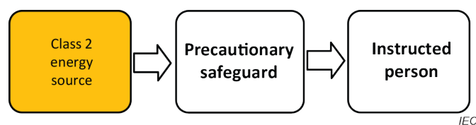
Figure 14 – Model for protection of an instructed person against a class 2 energy source
