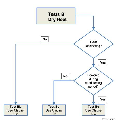
Figure 1 – Block diagram Tests B: Dry Heat
