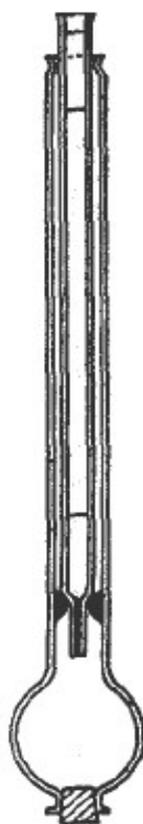
FIG. 2 VISCOMETER IN JACKET READY FOR TIME FLOW MEASUREMENT
