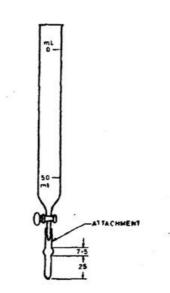
All dimensions in millimetres. Fig. 1 Burette with an Attachment
