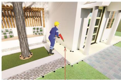
Drilling holes at 300mm distance
