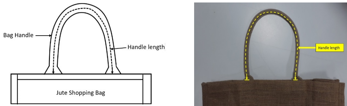
Figure 2: a) Schematic diagram of Bag handle length b) Real picture of bag handle length
