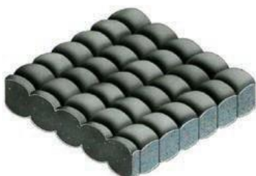
Figure C. Uniform Section Fabric form concrete Lining.
