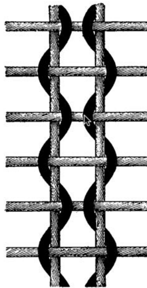
Figure 4: Full Leno weave structure showing alternating interlacement of doup ends (Shinn and Mckenna, 1930).
