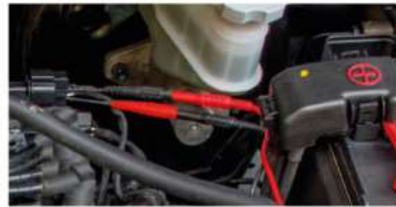
SIMULTANEOUSLY MEASURE BATTERY VOLTAGE AND VOLTAGE SUPPLY TO LAMBDA SENSOR.
