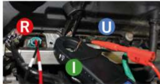
MEASUREMENT OF RESISTANCE, VOLTAGE AND POWER CURVES FOR INJECTION VALVES.
